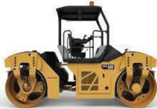
Fig-E8.2 (Solid drum type & excels on a variety of asphalt mix designs as well as other granular materials)
