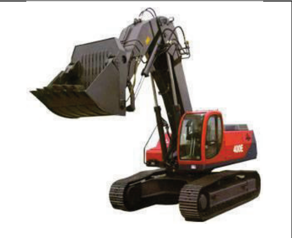
Fig-E 12: Crawler Hydraulic Excavator with Face Shovel
