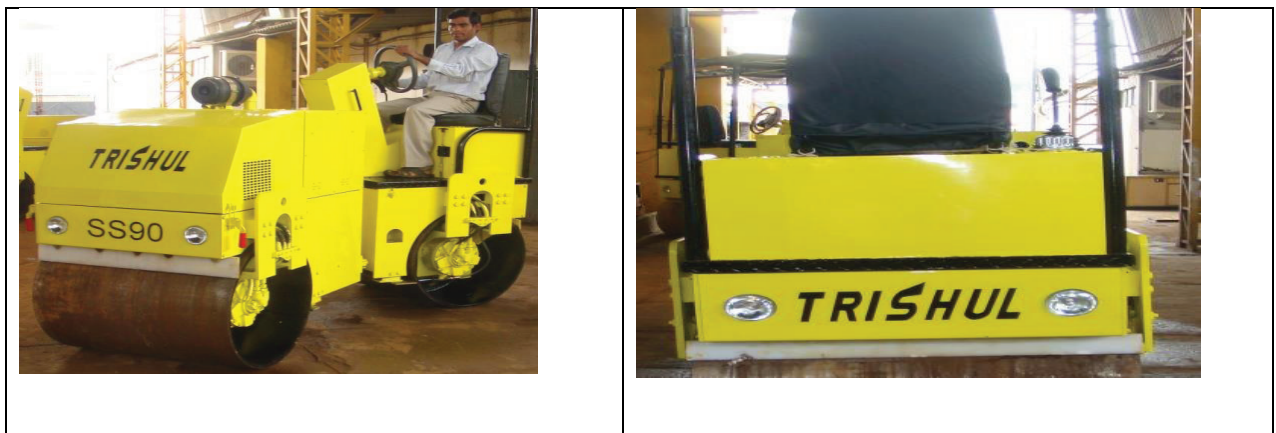
Fig-E6: Small Width Vibratory Roller (Drum width 90 cm)
