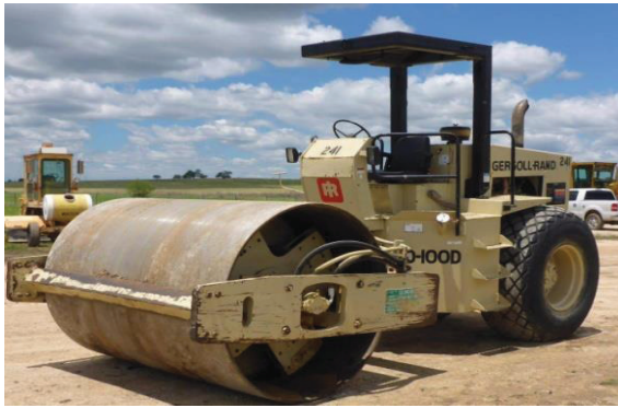
Fig-E9.1: (Drum Type & used for better gradeability)
