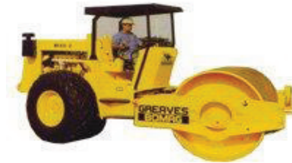
Fig-E9.3: Vibratory Rollers(Drum Type & used for better gradeability)
